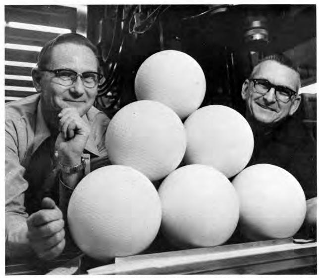
BUWLING BALLS they're not. They're 8" polyethylene spheres which will be criticality monitors near our nuclear reactors. Two kinds of dosimeters will fit into the small hole in each, with the sphere serving as neutron thermalizer. Dan Thompson (3313) has project responsibilities, but the precision machining was done by Keith Gawith (left) and his trainee, Jake Young (both 7146).
